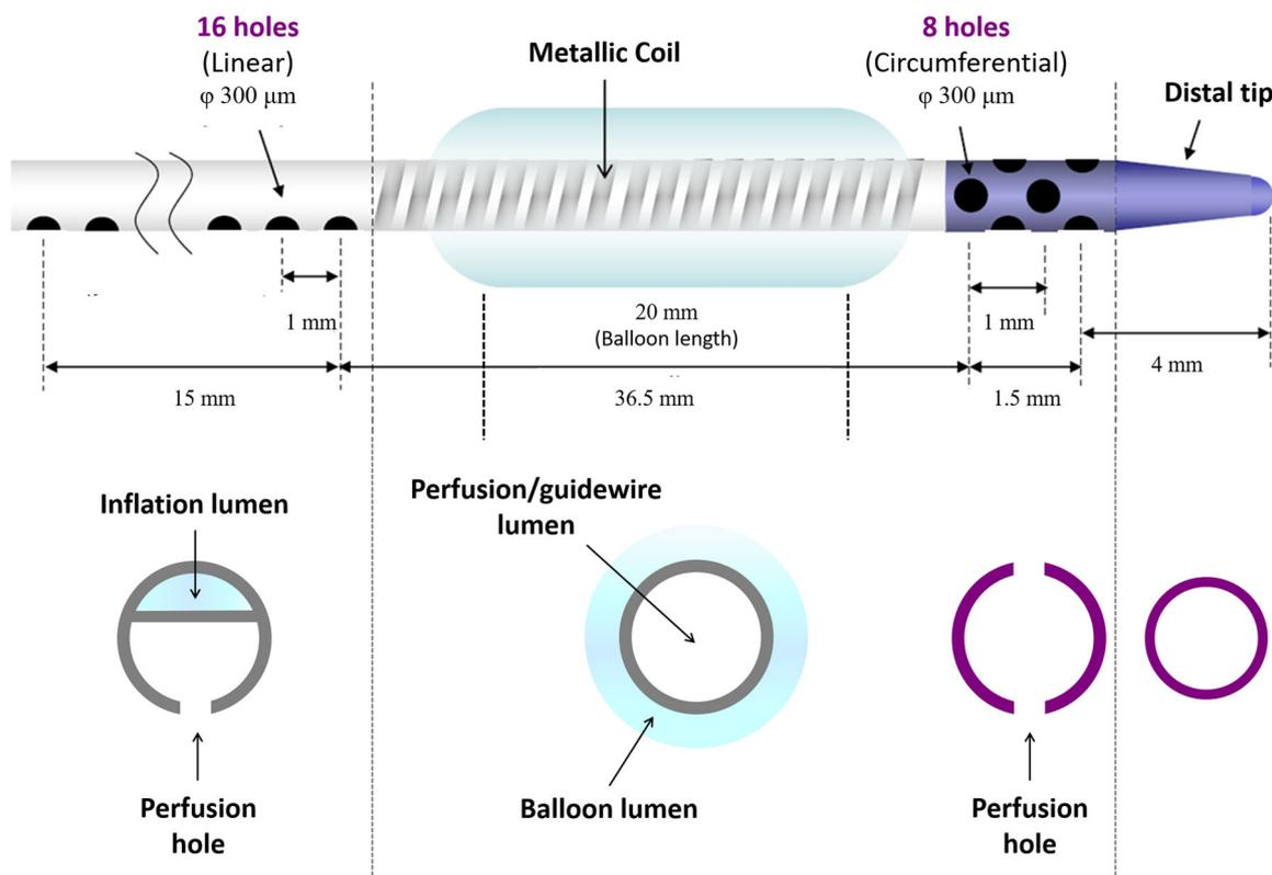
**FIGURE 1** | Structure of Perfusion Balloon. The perfusion balloon used in this study equips with 16 proximal and 8 distal perfusion holes ( $\phi 300 \mu\text{m}$ ), which allow coronary blood flow to pass from the proximal to the distal segment through the balloon shaft. [Color figure can be viewed at [wileyonlinelibrary.com](https://onlinelibrary.com)]
