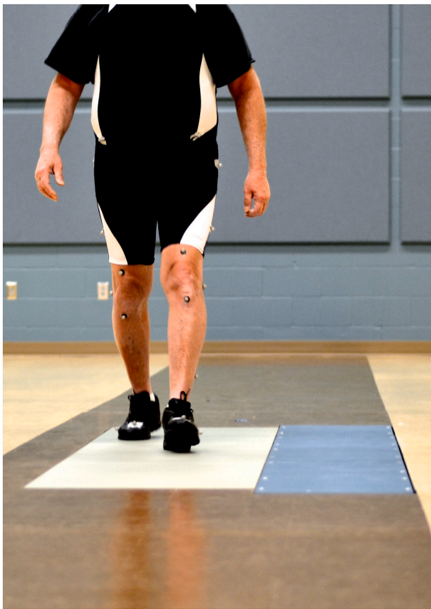
Fig. 1. In Fig. 1a, a patient with PAD is depicted walking on the force platforms with attached reflective markers. In Fig. 1b, a schematic view of the laboratory setup and the AFO utilized in this study is presented.
